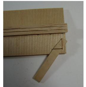
You can now glue the roof to the car. Apply glue sparingly to the tops of the sides and
