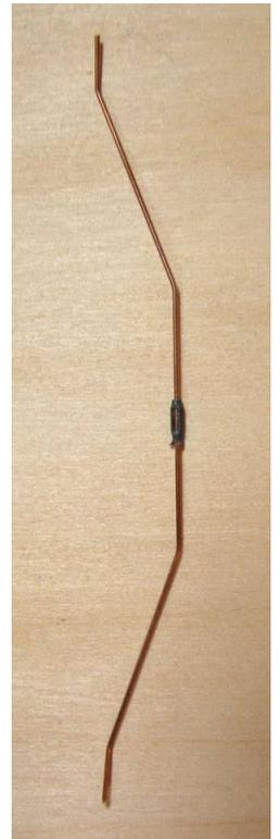
Put the rods back into the queenposts and over the bolsters, one at a time and hold them
