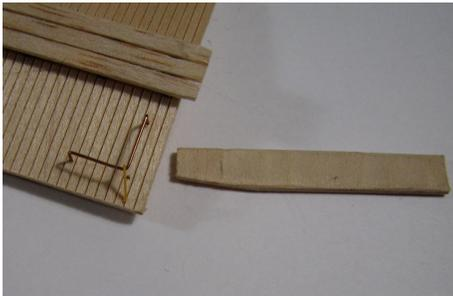
Now, install the corner roof grabs by sliding the eyebolt over the wire grab. Then push the two wires of the corner grab, part way into the roof, leaving the eyebolt loose at the corner. Now, lift the corner slightly and push the eyebolt
