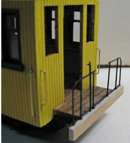
You can then add the brake wheel to the top of the single post. Place the wheel onto the pin shown and apply a small dab of CA. You may have to ream the hole in the wheel slightly (very carefully) to get it to fit over the post.
