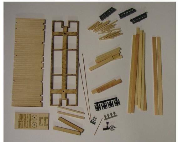
The first step is to drill the frame for the stake pockets. Included in the older kit is a hole location template. This must be lightly scribed along the fold lines and folded over the edges of the frame. Use some tape to hold it in place.
