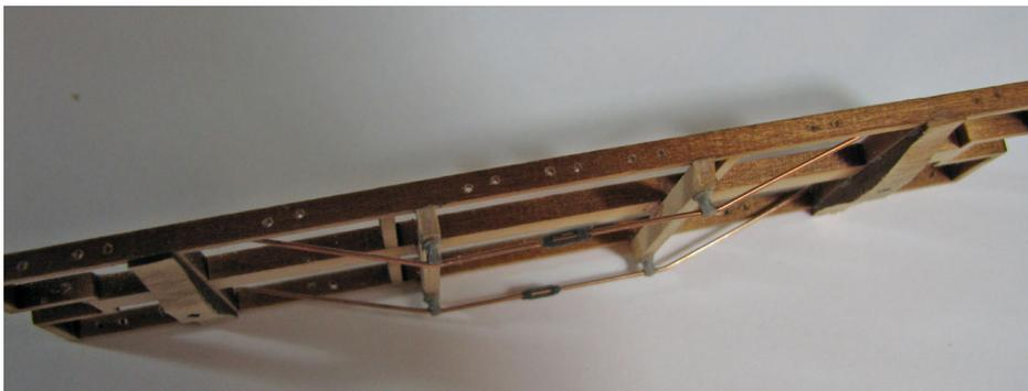
Lay the Truss Rods into the queen posts with the ends over the top of each bolster (with the frame upside down). Use CA to glue the truss rods into the queenposts and let it dry. Support the frame on a stand or block in the center while they dry. Once dry, turn the frame over and bend the ends down into the saw cut slots and apply
