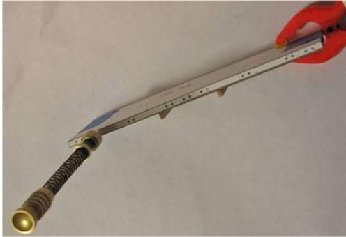
Use a #64 (.036) drill for the stake pocket holes and try to keep them straight across the frame. There is a small amount of play with this size hole to adjust the pockets when you glue them on. Drill the pair of end holes for the stirrups with a #71 (.026) drill.
