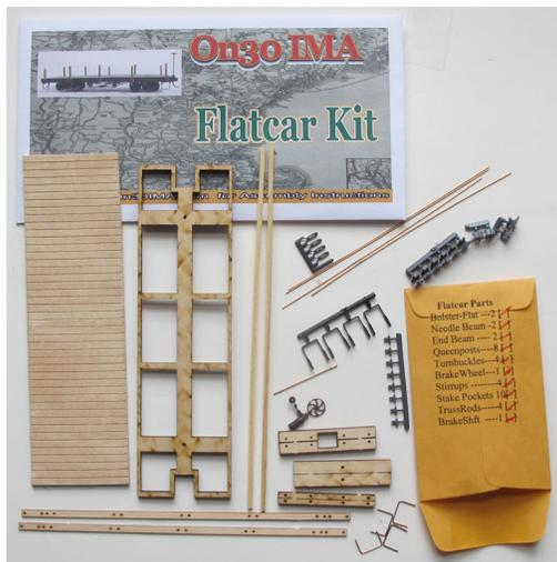
The first step is to drill the frame for the stake pockets. Included in the new kits are two plywood frame sides that are laser cut & pre-drilled for stake pockets and stirrup steps. All you have
