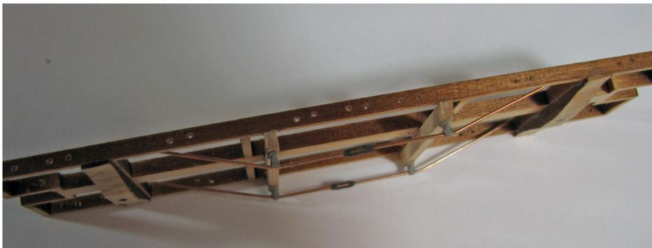
Lay the Truss Rods into the queen posts with the ends over the top of each bolster (with the frame upside down). Use CA to glue the truss rods into the queenposts and let it dry. Support the frame on a stand or block in the center while they dry. Once dry, turn the frame over and bend the ends down into the saw cut slots and apply CA to the end of each one. You may have to hold the end down while the glue sets or use an accelerator like I did.
