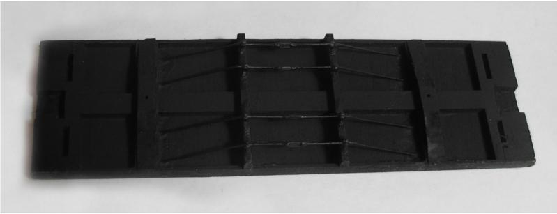
The kit includes both round bolsters or flat. If you choose to use the flat bolster, you need to taper the ends as shown. I simply carve them with my knife and sand as needed. I leave a small flat at the outside ends (not a chisel edge). Then, glue the Bolsters in place.
