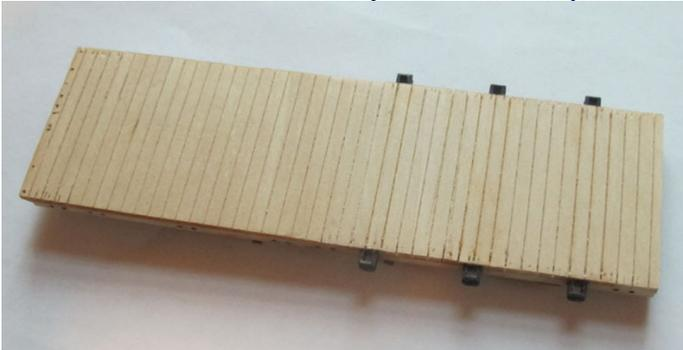
Sides assembled; note notches I cut in the end tops for a long roof beam on each side.
