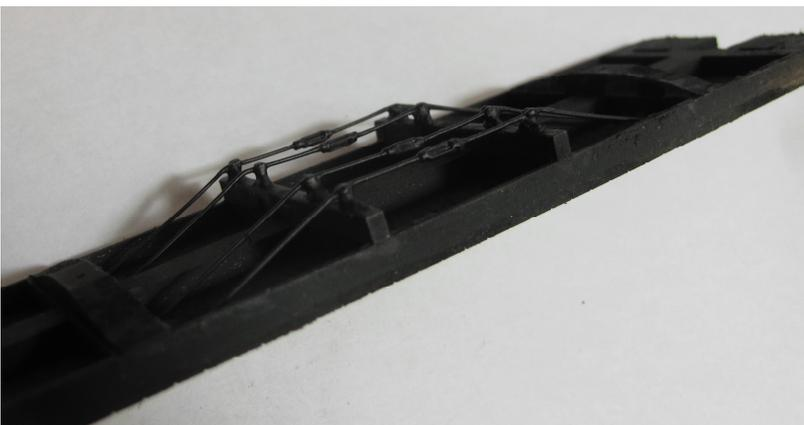
Lay the Truss Rods into the queen posts with the ends over the top of each bolster (with the frame upside down). Use CA to glue the truss rods into the queenposts and let it dry. Support the frame on a stand or block in the center while they dry.
