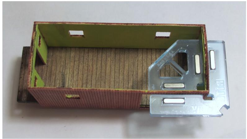
Glue one side to the edge of the frame, locating it central to the floor length (equal number of boards at each end). Make sure the bottom edge of the side is flush to the bottom of the frame. After that is set up, glue the ends in place with a fine line of glue at the corner joint. Those right angle magnetic clamps from Rite Way are expensive but a great tool.
