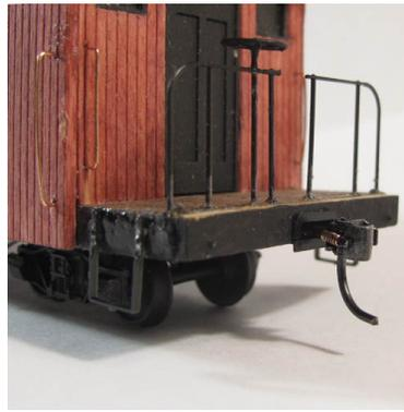
Now glue the 4 NBWs into the two end beams. Trim them flush on the back side and glue the end beam to the end of the car. An alternate method is to glue the end beam to the car and then drill out the frame to accept the NBWs. Next, glue the stirrups to the side of each platform. I used a #70 drill and made a drill template (to match the stirrup pins) to drill the holes in the frame, just under the floor.
