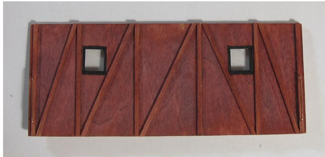
**ALTERNATE ASSEMBLY:** If you purchased the outside braced kit with plain sides, you can install the bracing now. Cut the 12 vertical braces to length for the sides and then the 10 diagonals to fit between them. **Note: The vertical braces MUST be cut from the shorter bundle and the diagonals from the longer bundle of stripwood.**
