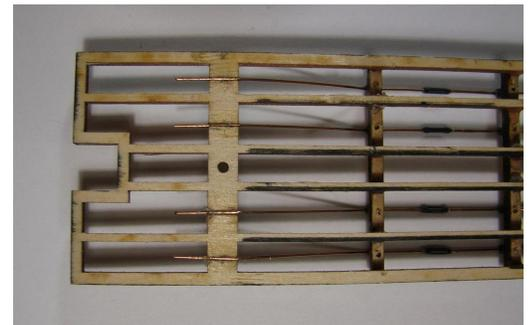
After the glue dries, trim the trussrod ends with your cutting pliers.
