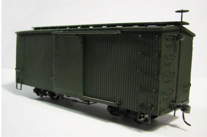
After that dried, I used the airbrush to paint the car CN Green. Although this was a new bottle of airbrush paint, it took me a couple tries to get a half way decent finish. I'm new to the airbrush so maybe my next one will come out better. I sprayed the doors separately, taking care not to get paint on the running edges.
