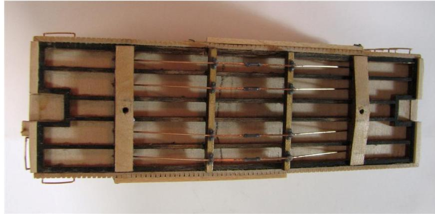
Glue the full bolster to the frame bottom. Drill the bolster with the appropriate hole size for your truck screws using the hole in the frame top as a guide.
