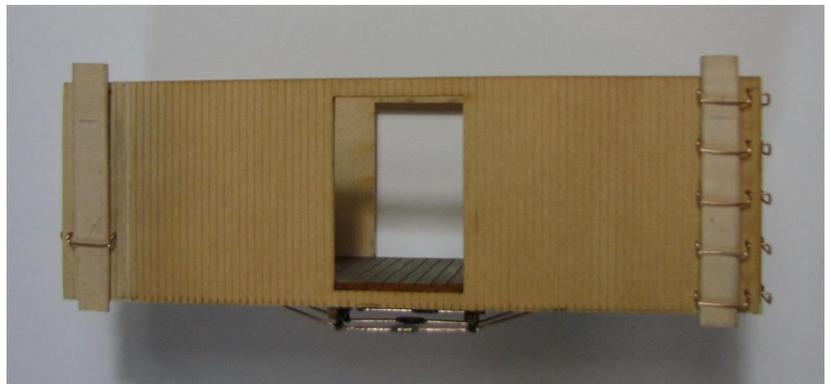
Insert the wire grabirons into the holes, one row at a time. Slide a 1/16" spacer behind them and hold in place (I use tape). Now apply a drop of CA to the back of each grab wire. I sprayed with accelerator to speed up the process.
