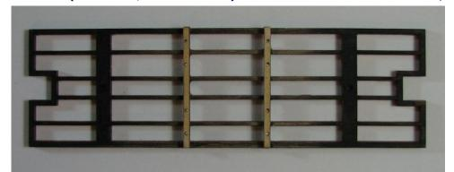
you, making sure the beams are square to the sides (use a small square). Now drill the needle beams to accept the queenposts. The hole location is marked along the centerline of each needle beam and should be drilled with a #58 - #60 drill (.042"
