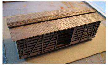
ends and place the roof down. Make sure the reveal is equal all the way around under the roof edges. Adjust as necessary and hold down with rubber bands. Do not put them on too tightly as it may warp the roof or sides. Now add the three walk boards to the roof. Apply glue sparingly to each roofwalk support and place the boards down, one at a time, keeping them aligned with the support edges and straight.
