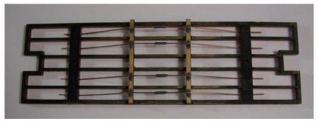
After the glue dries, trim the trussrod ends with your cutting pliers.
