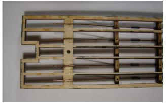
tight into the queenposts (I used my small spring clamps). From the top of the frame, push the rod into the slot, hold it there (I used a small clamp on the extended end) and apply CA (super glue). Glue both ends and each rod one at a time. If the rod moves out of the queentpost, that means they are over bent and should be flattened so they will remain in the QPs,
