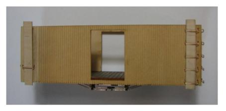
Insert the wire grabirons into the holes, one row at a time. Slide a 1/16" spacer behind them and hold in place (I use tape). Now apply a drop of CA to the back of each grab wire. I sprayed with accelerator to speed up the process.
