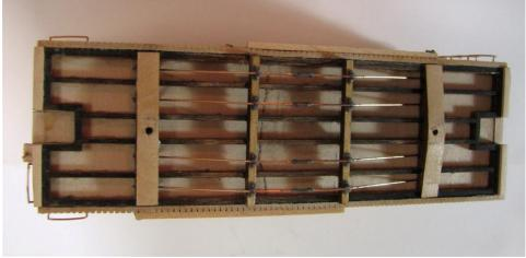
Glue the round or full bolster to the frame bottom. Drill the bolster with the appropriate hole size for your truck screws using the hole in the frame top as a guide.
