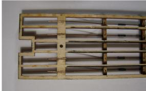
After the glue dries, trim the trussrod ends with your cutting pliers
