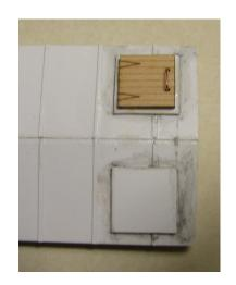
The Hatch Frames are square and can be glued to each corner as shown. If you decide not to use the corner roof grabirons, the hatch base can be located to cover the holes in the roof. Otherwise, the base must be kept back, just flush to the holes to allow installation of the corner grabs. The Hatches can then be glued on top of that. If you want the hatches to be open, you can glue them in that position. The latest kits include both a hatch frame and the hatch.
