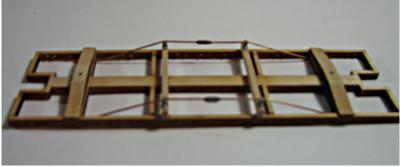
An alternative to using the truss rod material is to use either a .022" fishing line or jewelry beading wire and feed it through holes drilled into the end beam and glued. The newest kits have a drilled End Beam and NBWs for you to use after the floor is installed.
