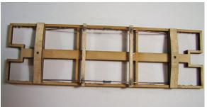
The kit includes flat bolsters that you need to taper the ends as shown. I simply carve them with my knife and sand as needed. I leave a small flat at the outside ends (not a chisel edge). Then, glue the Bolsters in place. Next, drill the bolster for the truck screws using the top side hole of the bolster as a guide.
